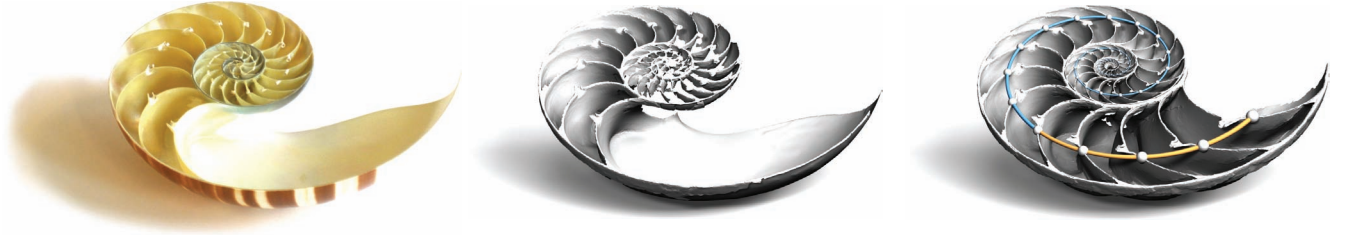
Figure 16: Model repair and geometry synthesis for a scan of a chambered nautilus shell. From left to right: photograph of original model, input data consisting of 72 registered laser scans, repaired model with additional synthesized elements indicated in orange.
