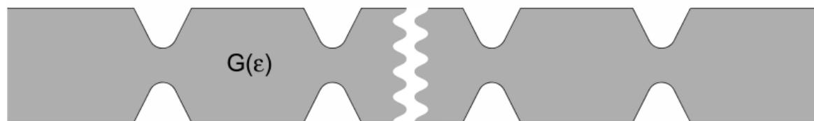
Figure: Waveguide  $G(\varepsilon)$  with  $n$  equal resonators
