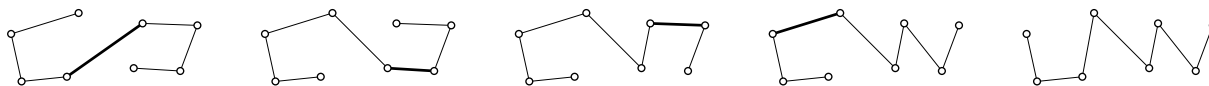
Figure 2: Flipping to an x -monotone path in four steps. In every step the bold edge is flipped.
