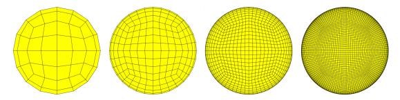
Figure 11: Frontal view of the graded meshes used for the Poiseuille flow problem.
