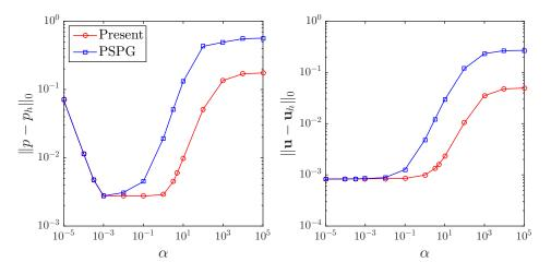
Figure 7: Kovasznay benchmark: error with respect to stabilisation parameter.
