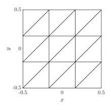
Figure 4: Kovasznay benchmark: coarsest mesh used in the refinement study.
