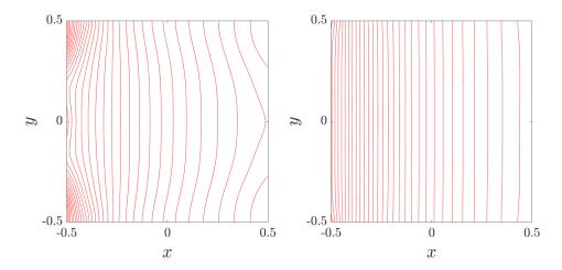
Figure 8: Kovasznay benchmark: pressure isolines for PSPG (left) and present formulation (right).
