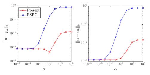
Figure 10: Poiseuille flow: error with respect to stabilisation parameter.
