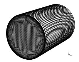
Figure 9: Poiseuille flow: graded mesh used for the first test case.
