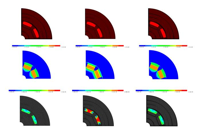
Figure 4: Initial configuration, objective value  $2.33 \cdot 10^{-8}$ . 1st row: level set function. 2nd row: B-field ( $||B|| = ||\operatorname{curl} u||$ ). 3rd row: topological derivative. Left column: bottom. Central column: center. Right column: top.
