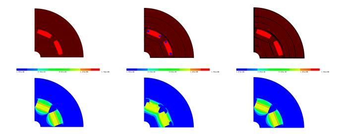
Figure 5: Improved configuration (after 1 iteration, objective value  $4.68 \cdot 10^{-9}$ ). 1st row: level set function. 2nd row: B-field ( $||B|| = ||\operatorname{curl} u||$ ). Left column: bottom. Central column: center. Right column: top.
