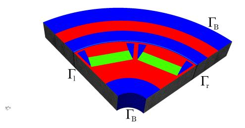
Figure 2: Three-dimensional model of electrical machine D with ferromagnetic subdomain  $\Omega$  (red), permanent magnet regions  $\Omega_2$  (yellow), air subdomain D\( $\Omega \cup \Omega_2$ ) (blue) with air gap region  $\Omega_g$  (light blue), lateral boundaries  $\Gamma_l$ ,  $\Gamma_r$  and inner and outer boundaries  $\Gamma_B$ .
