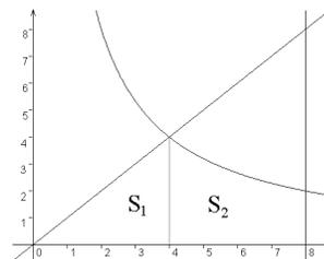
$$\begin{aligned} I &= \iint_{S_1} x^2 \, dx \, dy + \iint_{S_2} x^2 \, dx \, dy = \int_{x=0}^4 \left\{ \int_{y=0}^{\bar{y}=x} x^2 \, dy \right\} dx + \int_{x=4}^8 \left\{ \int_{y=0}^{\bar{y}=\frac{16}{x}} x^2 \, dy \right\} dx \\ &= \int_{x=0}^4 \left\{ x^2 y \Big|_{y=0}^{y=x} \right\} dx + \int_{x=4}^8 \left\{ x^2 y \Big|_{y=0}^{y=\frac{16}{x}} \right\} dx = \int_0^4 x^3 \, dx + \int_4^8 16x \, dx = \frac{x^4}{4} \Big|_0^4 + 16 \frac{x^2}{2} \Big|_4^8 = 448 \end{aligned}$$
